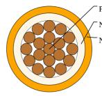
Plain copper conductor NBR modified PVC insulation NBR modified PVC sheath
